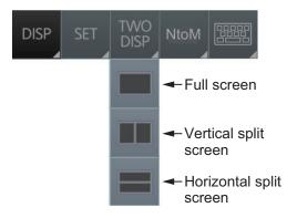
The example below shows the vertical split screen. The active display can be switched by clicking an [ACTIVE] button at the top of the display. The dividing line between the main and sub views cannot be moved.
