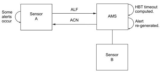
If the HBT sentence is not received from equipment within the prescribed time interval, the alert processed as responsibility transfer alert is made active and the "System communication fail" alert is generated.
