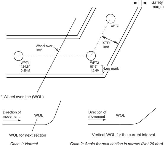
Case 2: Angle for next section is narrow (Not 20 deg)
