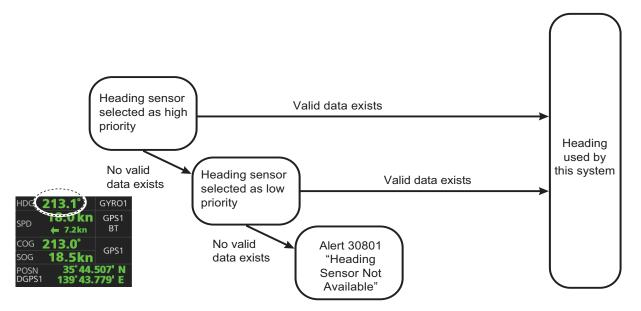
SOG/COG used by the system is shown at the top-right position on the chart display. In the example below, COG and SOG are from chosen position sensors and this is indicated with the text "GPS\*" or "LOG\*" (\* is the number of sensors).
