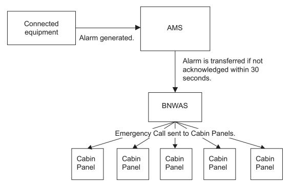
**Note:** The transfer of Alarms can be stopped (when in port, etc.) by setting the system in Silent mode. See section 1.4 for details.
