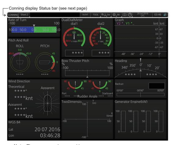
**Note:** The cursor can be moved between the main monitor and a sub monitor and vice versa if the sub monitor is configured to show the Conning display. Push the scroll-wheel until the cursor moves to the other monitor.
