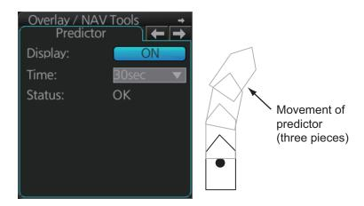
The Predictor is updated every three seconds internally and the status of the predictor is shown with [Status] as shown in the table below.
