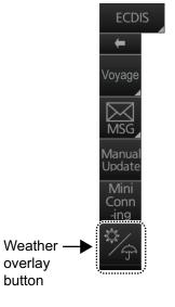
When the weather overlay is made active, two weather overlay dialog boxes appear, [Weather Overlay Control] and [Weather Overlay]. The [Weather Overlay Control] dialog box selects and plays back weather data files. The [Weather Overlay] dialog box controls what weather information to display and how to display it.
