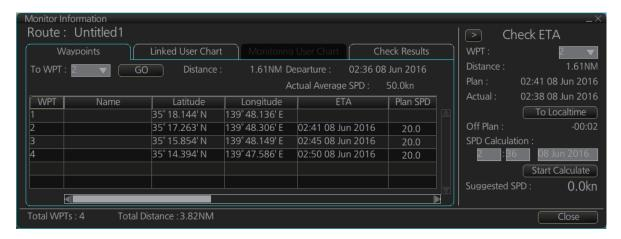
**Note:** A route cannot be opened if its planned settings are different from its navigation settings. The reason is given on the [Select Route] dialog box. In this case, open the route in the Voyage planning mode and click the [Check Route] button, on the [Alert Parameters] page. Adjust the route as necessary.
