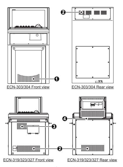
It is recommended to have a qualified technician clean and check the air filters when conducting routine service and maintenance. If the air filters require replacement, consult your dealer and quote the following details:
