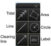
4. Click the desired object (button) on the palette. The [Tidal], [Line], [Clearing line] and [Label] buttons have multiple choices. Right-click the respective button to show a context sensitive menu. The choices available for each object are shown below.
