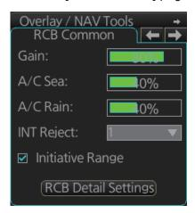
2. [Gain] adjusts the strength of the radar signal. Adjust the gain so that the background noise is just visible on the screen. If the gain level is too low, weak echoes may be missed. On the other hand, if the gain level is too high, the strong background noise can hide weak targets.
