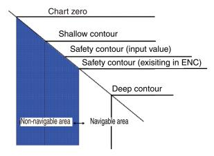
In the two-color presentation, unsafe water is shown in blue and safe water is shown in white. The safety contour is used to qualify unsafe water (depth shallower than safety contour) and safe water (depths deeper than safety contour).
