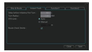
[Delay before Initiating First Turn]: Set the number of seconds (30 - 600 seconds) to wait before initiating the first turn in the simple route.
