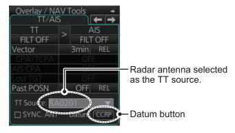
To automatically select the radar currently displaying radar echoes as the TT source, check the [SYNC. ANT] box on the [TT/AIS] page in the [Overlay/NAV Tools] box.
