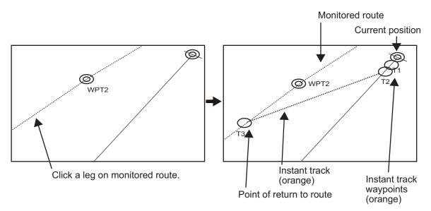
The system uses ship position, speed and final waypoint to create a track. The track is also checked for hazardous objects and the like against the chart alerts.
