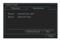
For the [Back to Track] mode, the instant track mode is canceled when the vessel returns to the monitored route. The instant track is greyed out to show that it is inactive.
