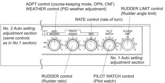
**ADPT control**: Select OPN (Open Sea) when economical operation is required. The course is followed with the least necessary steering, allowing a little meandering when; for example, sailing on the open sea.
