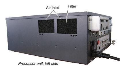
If the filter appears brittle and leaves residue on your hands when dry, replace the filter.
