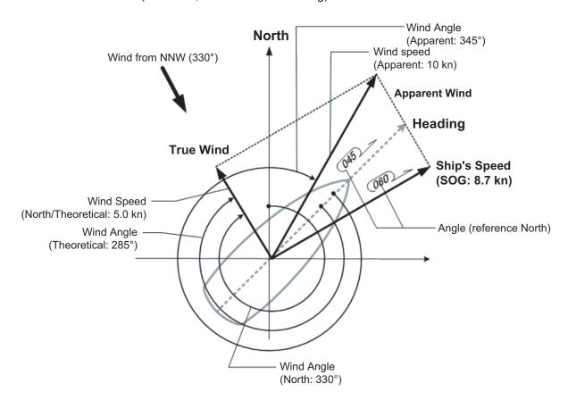
Apparent, North (true wind referenced to North), Theoretical (true wind referenced to heading) may be selected from the [Other Sensor Settings] menu. If the wind indication is not accurate; for example, the wind is blowing from the North but the wind direction displays otherwise, check if the format is Theoretical. If it is, switch to another format.
