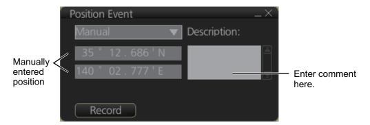
The [Position Event] window shows the position at the moment the [Record] button is clicked. The position is recorded to the [Voyage] log.
