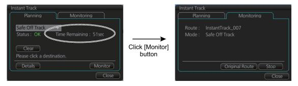
The vessel follows the instant track route in the same method as a monitored route, which is greyed out to indicate it is inactive. For the instant track route connected to a monitored route, the previous instant track route is also greyed out to show it is inactive. Any additional instant track routes are erased.
