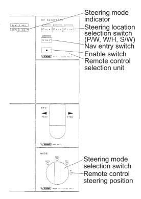
**Note 2:** When you select the RC mode, select "RC" in one motion. Do not stop at any of the secondary positions on the switch, to prevent loss of the TCS. If the TCS is lost, first check that the rudder is centered then restore manual steering (HAND) at the autopilot. Restart TCS (GoAW) at the ECDIS then reselect RC.
