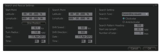
2. Enter your start point. To enter current position, click the [Ship Position] button. (The start point can also be entered directly on the screen. Put the cursor on the start point, right-click the chart to show the context-sensitive menu shown below then click [Set start point].)
