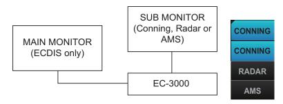
Dual monitor configuration and Display mode button
