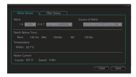
Wind: Select wind unit, wind reference, and wind source. See section 18.9.
