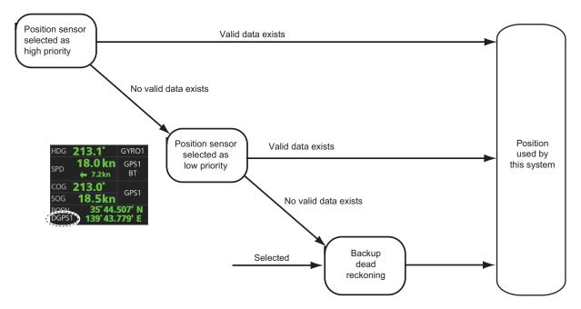
If the system changes the source of position because of lost sensor data, the system immediately generates the Alert 30602 "Position Source Change".
