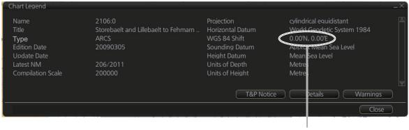
WGS 84 shift indication (0.00'N, 0.00'E means no shift)
