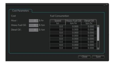
At the [Cost] window, enter the cost/hour and cost/ton for heavy fuel oil and diesel oil. At the [Fuel Consumption] window, define the fuel consumption figures for up to 12 different speeds. Before entering the data, plot the data on a graph, like the one shown below. Use a second graph if, for example, diesel oil consumption is different from that of heavy fuel oil. Reset the power to effect the settings.
