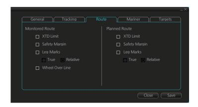
XTD Limit: The distance from the centerline to one side of the nav lane. Safety Margin: The distance from one side of the channel limit to the safety margin distance.
