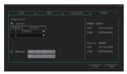
**Sensor**: Name of sensor used. Position sensors have priority in order of accuracy. When a sensor is changed, the Alert 30602 "Position Source Change" appears. **Manual**: When a sensor cannot be used, select [Manual], then enter position manually.
