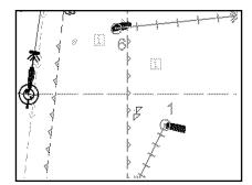
Equal gyro value at radar and ECDIS
