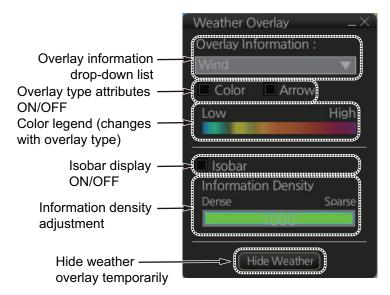
tion] drop-down list. The choices are [Wind], [Temperature], [Cloud Coverage], [Precipitation Rate], [Wave], and [Ocean Current]. (The weather data file must contain the data selected in order to display it.)
