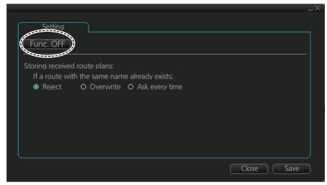
2. Click the function button (circled in the figure above) to change its label to read [Func ON] (route transfer is enabled) or [Func. OFF] (route transfer is disabled) as required.
