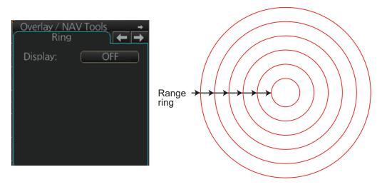
The interval between rings changes with the chart scale, as shown in the table below.
