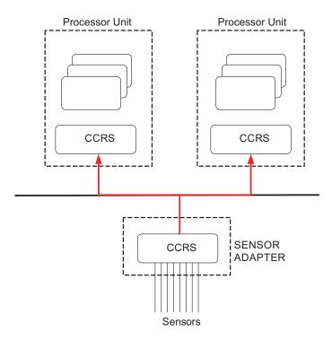
The CCRS processes IEC 61162-1 and IEC 61162-2 data sentences. No other types of data (video signals, etc.) are processed.
