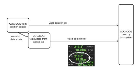
Speed used by the system is shown at the top-right position on the chart display. The figure below shows the source of water speed is used for drift calculation.
