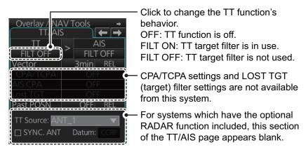
**Note:** The TT symbols, AIS symbols and radar displays can be hidden. Click the [CLEAR RADAR] button on the Status bar to hide those displays.
