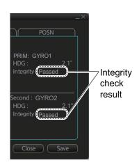
**Note:** The integrity results appear in the [Local Sensor Setting] and [System Sensor Setting] menus only if the menu item [Color of own ship's information(TEXT) will be changed by result of integrity check] is checked during installation.
