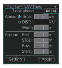
2. Set the ahead time or distance and ahead width, referring to the figure below. Also, set the "Around" figures: port, starboard, bow and stern check distance. The reference point is the conning position (CCRP).
