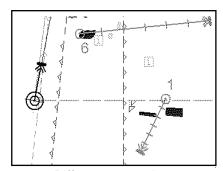
Different gyro value at radar and ECDIS
