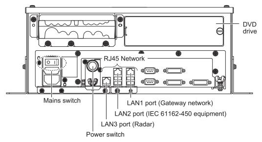
**Note 1:** Do not operate the system with a medium inserted in the DVD drive when its use is not required, to prevent damage to the drive and medium. After use of a medium is completed, remove the medium from the drive and store it in its case.
