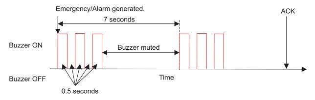
IEC 62288 Ed.2 mode, emergency/alarm priority buzzer
