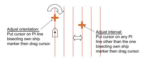
How to adjust orientation and interval, multiple PI lines
