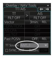
To automatically select the radar currently displaying radar echoes as the TT source, check the [SYNC. ANT] box on the [TT/AIS] page in the [Overlay/NAV Tools] box.
