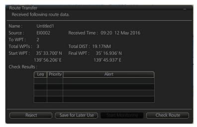
Select the appropriate handling for the received route from the buttons at the base of the [Route Transfer] window.
