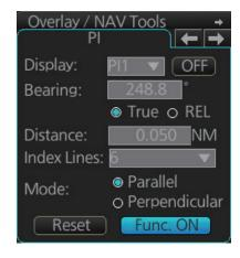
The bearing can be set two ways: with the scrollwheel or dragging the PI line on the screen.
