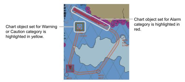
For this function, the ECDIS utilizes the chart database (S57 charts) stored on the SSD in SENC format. Note that the ECDIS calculates dangerous areas using the largest scale chart available, which may not be the visualized chart.
