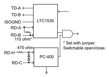
Processor Unit, Sensor Adapter: IEC 61162-2/1 input/output
