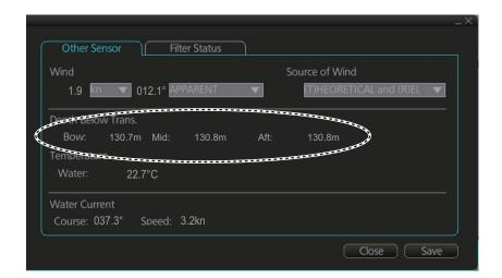
The system displays depth value as depth below the transducer. If required, you can get an alert when the measured depth is less than the "Echo Alarm Limit" setting at the [UKC] page in the [Overlay/NAV Tools] box. The system generates the Alert 30801 "Depth Limit".
